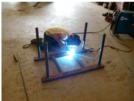
Maintenance staff fabricating a sturdy frame
